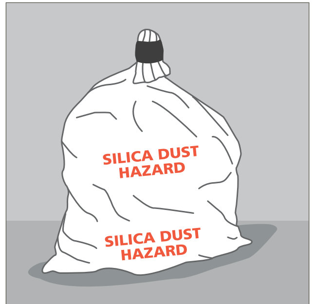
Figure 16: Waste contaminated by silica dust needs to be bagged and labelled
