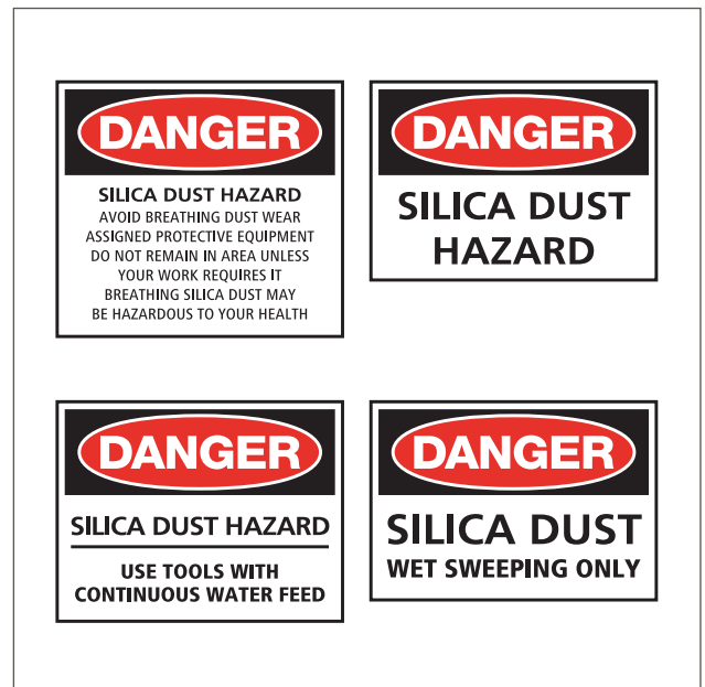
Figure 13: Silica dust hazard warning signs
