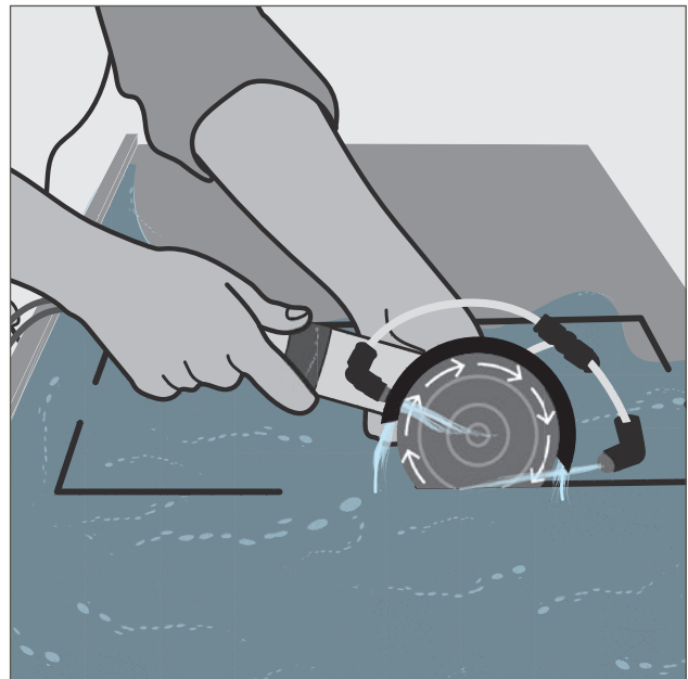
Figure 7: Good spray control – guarding deflects water down towards the slab
