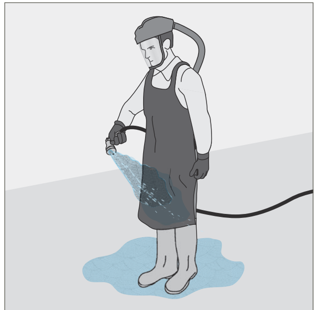
Figure 15: Spray down with a low pressure hose to decontaminate PPE
